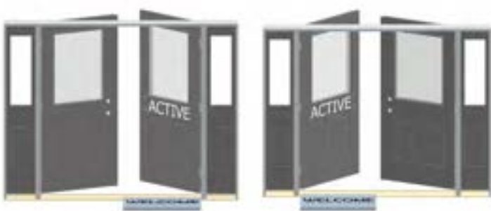
SOXS (Sidelite-Fixed- Operable-Sidelite, HLIS)
